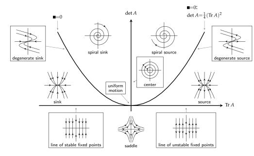
Poincaré Diagram: Classification of Phase Portaits in the  $(\det A, \operatorname{Tr} A)$ -plane
